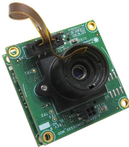
Fig-1: See3CAM_30 USB 3.0 Camera with Liquid Lens
