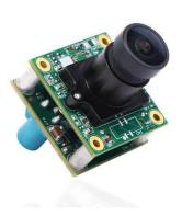
NeduCAM25 is the first product launched in the NeduCAM series – a portfolio of FPD-Link III cameras from e-con Systems. NeduCAM25 is based on onsemi®'s AR0234 sensor. The global shutter feature of this camera helps to capture fast-moving objects without any rolling shutter artifacts. It uses the FPD-LINK III interface with shielded coaxial cable for reliable transmission of both power and data up to a distance of 15m with low latency.
