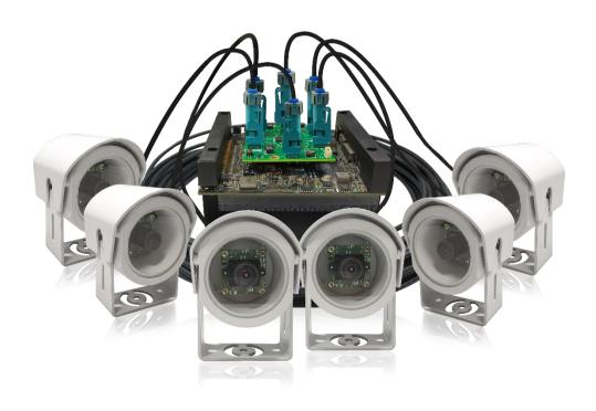
Designed and developed to work seamlessly with the NVIDIA platform, STURDeCAM25 has off-the-shelf support for the **Jetson development kit** and **Connect Tech's Rogue** platform based on Jetson AGX Xavier, Rudi AGX platform based on Jetson AGX Xavier, and Rudi NX platform based on Jetson Xavier NX. This enables rapid prototyping and faster deployment of vision enabled products.
