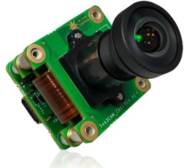
High Signal to Noise ratio of this camera helps to produce videos and images with low noise even in poor lighting conditions. It comes with an M12 (S-mount) lens which allows customers to choose the lens of choice according to their application needs.
