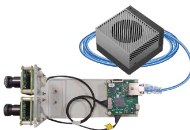
Figure 2: Holoscan camera solution integrating cameras with NVIDIA platforms through Lattice FPGA
