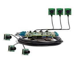
This multi-camera solution allows connecting up to 6 cameras (MIPI or GMSL2 or a combination of both) simultaneously. e-con Systems' cutting-edge camera solution, along with Qualcomm's high compute power of 15 TOPS, low power consumption, and thermal dissipation, is the perfect choice for applications such as drones, delivery robots, and autonomous shopping systems.
