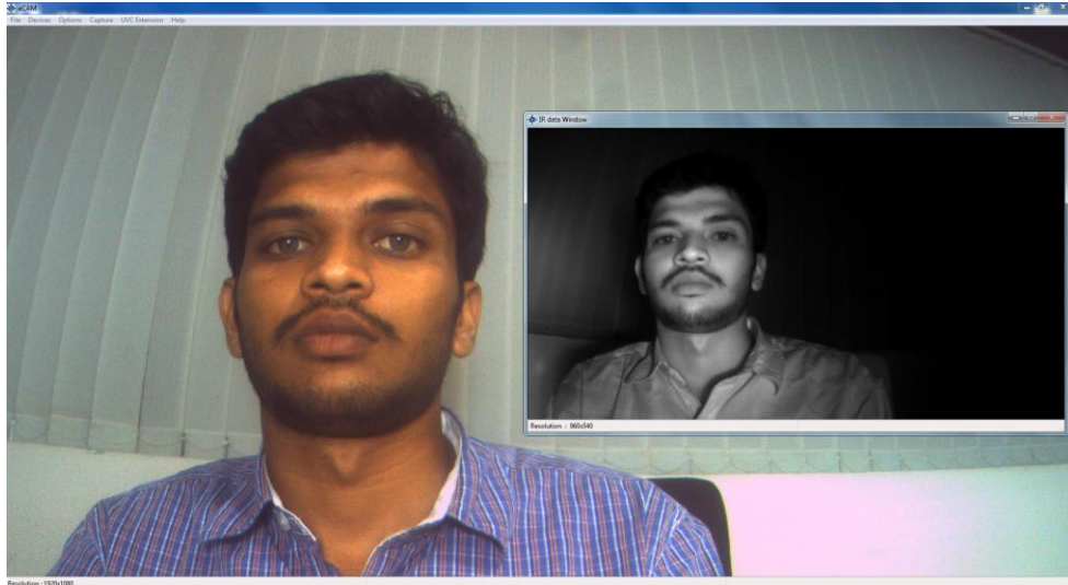
Fig: e-CAMView Application showing RGB video and IR video from See3CAM_CU40
