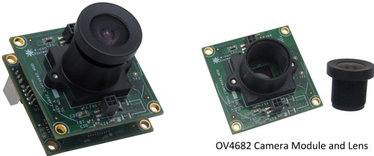
Fig: See3CAM_CU40 USB 3.0 RGB-IR Camera with M12 Lens
