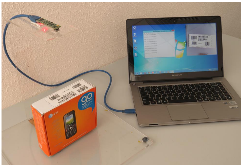
Fig: See3CAM_80 Capturing the Barcode and decoded by Spica
