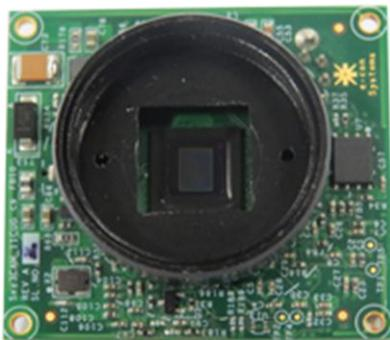
**Figure1: See3CAM\_11CUG – 1.3 MP camera with CS Mount Lens holder**
