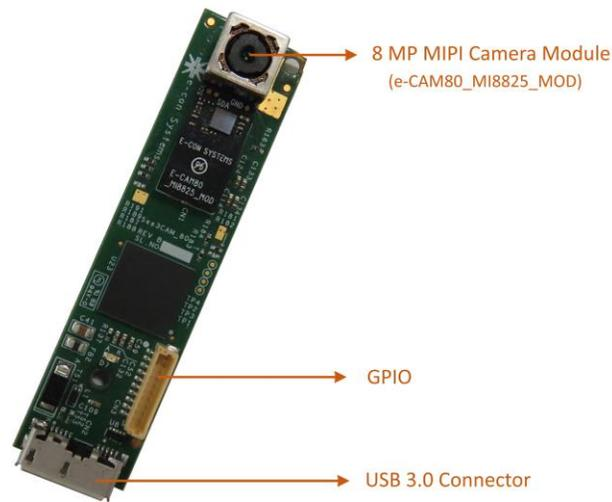
Fig: See3CAM\_80 camera with e-CAM80\_MI8825\_MOD module
