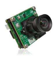
Further, See3CAM\_CU135M is a high-resolution camera with a resolution of 13MP. This helps to capture images with great details, which is a critical feature in microscopic applications. This 4K monochrome camera streams video data in Full HD @ 60 fps & 4K @ 30 fps with output formats of Y8 and Y16. Also, it has an S-mount lens holder which allows customers to choose and use their own optics.
