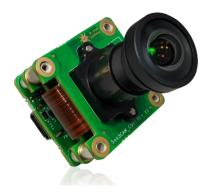
High Signal to Noise ratio of this camera helps to produce videos and images with low noise even in poor lighting conditions. It comes with an M12 (S-mount) lens which allows customers to choose the lens of choice according to their application needs.
