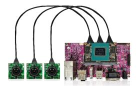
This multi-camera solution comes ready to be evaluated with the NVIDIA® Jetson Xavier<sup>™</sup> NX development kit and Diamond System's FLOYDNX carrier board with the necessary software. The solution allows customers to connect up to three 4-lane MIPI camera modules on the FLOYD carrier board housing NVIDIA Jetson Xavier<sup>™</sup> NX. This MIPI camera module can stream 18MP at 13 fps with 4-lane configuration.
