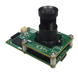
**FSCAM\_CU135** has a powerful 13 MP resolution-based 1/3.2-inch AR1335, a 1.1-pixel BSI CMOS image sensor from ON Semiconductors™ and is equipped with a S-mount (M12) lens holder that enables customers to pick a lens of their choice. It is powered by the Xilinx Spartan® series FPGA - with on-board DDR memory for storage.
